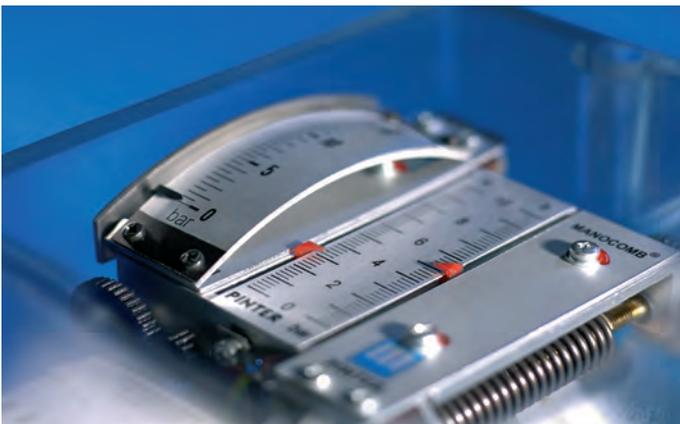
**Pressure Switches** | Signal elements which are used for pressure measuring in pressure lines for gases, vapours, liquids or suspensions. The switch points are transformed into a binary electric or pneumatic output signal which is necessary for the control and regulation of processes, e.g. safety and alarm devices.
