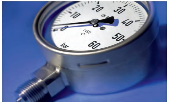
**Pressure Gauges** | Mechanical pressure indicators. The actual process pressure acts on a measuring element and deforms it. The deformation is converted into a 270° rotating motion by the attached movement. Due to the electricity-free function, pressure gauges even remain fully functional in most total damage occurrence.
